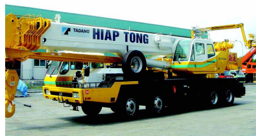
MOBILE TRUCK CRANE
