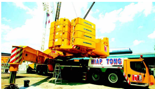
ALL TERRAIN CRANE
